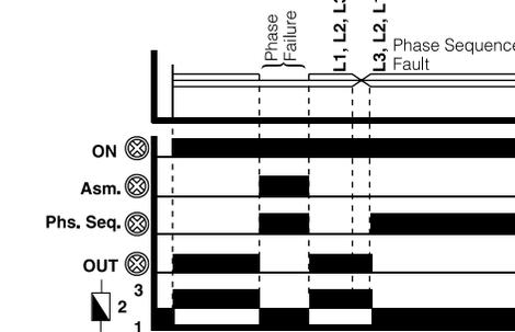
Phase Sequence Fault Function Diagram
